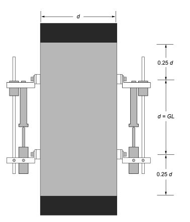
Figure 2—General Schematic of Gauge Points (not to scale)
