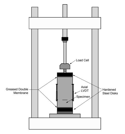
Figure 1—General Schematic of Dynamic Modulus Test
